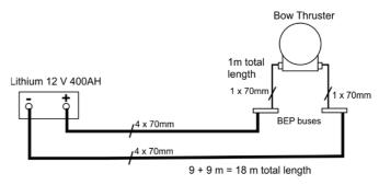
a) There is a total of about 18 meters of cable (+ve plus -ve) between battery and the BEP buses at the bow thruster. The cables are made up of 4 x  $70 \text{mm}^2$  ( $70 \text{mm}^2 = 0.000281 \ \Omega/\text{m}$ ).
