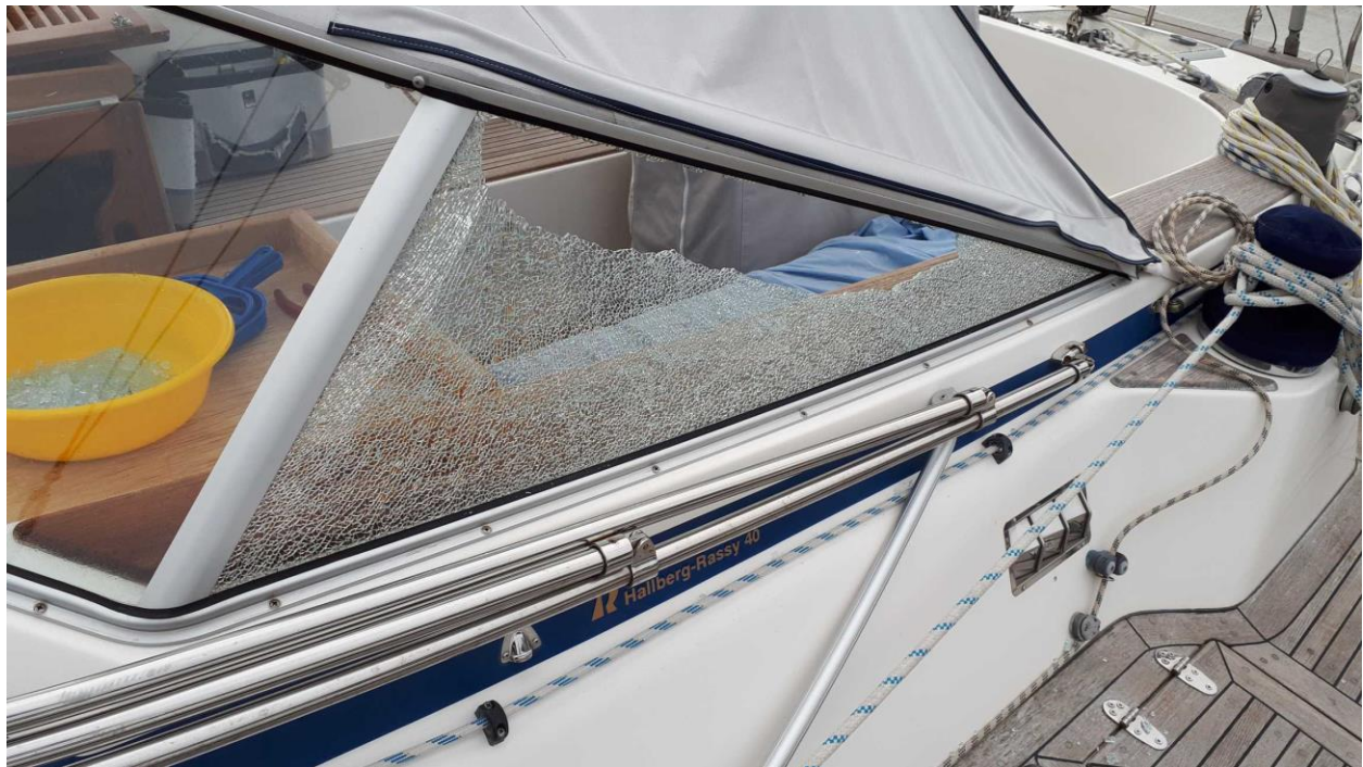
The shattered glass pane after handle was simply taken off
