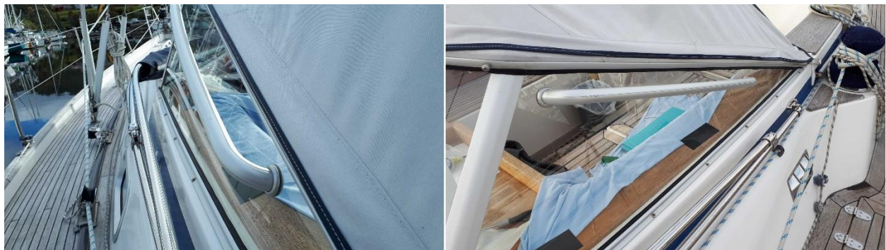
The new toughened glass pane fitted - note its slight curvature as it was slightly bent to fit into the curve of the aluminium frame
